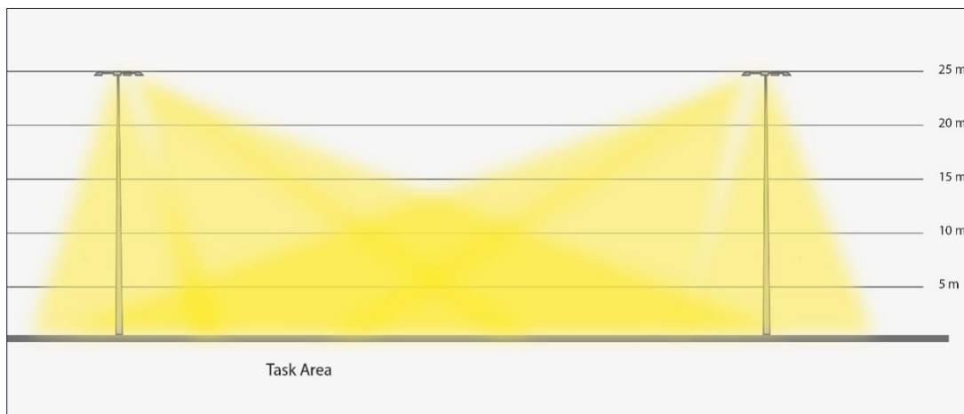
Inset 5.11 Wide area lighting arrangement
